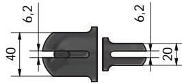
PA with clevis Max. static load 4700 N Max. load 3100 N (gear ratio 1:24)
